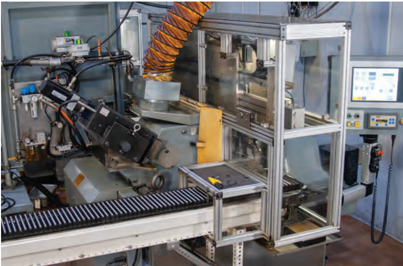
The Grinding Department is where all studs are centerless ground to ensure that they are concentric and straight.
