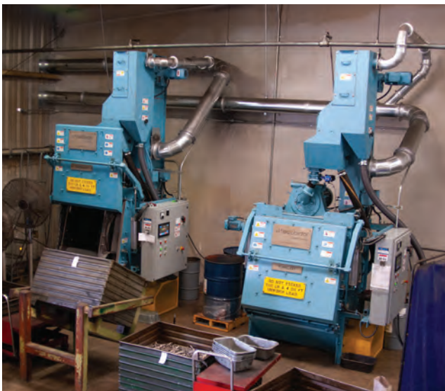
Fasteners are shot-peened to improve fatigue life.
