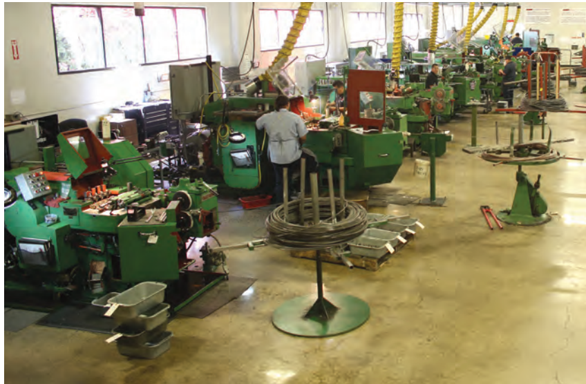
ARP's bank of cold-headers can handle material up to 5/8" diameter and form bolts in a multi-phase operation.
