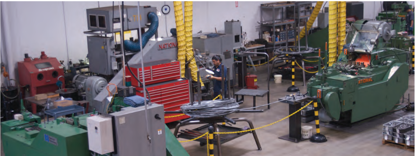
Powerful cold-forging equipment is used to make ARP's hex and 12-point nuts. Multi-stage dies are employed to precision-form the finished "blanks."
