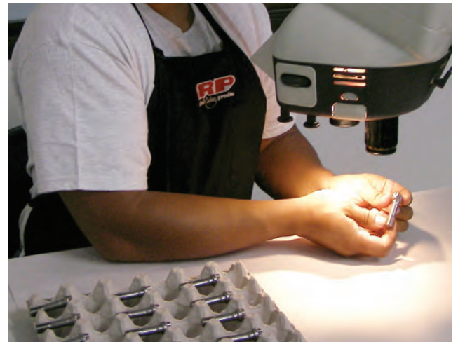
High powered magnifiers are used to carefully inspect critical components. ARP's quality control team is relentless!
