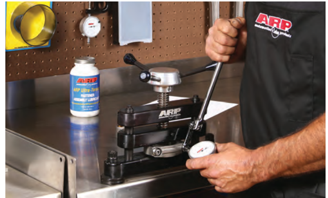
A rod bolt stretch gauge is one of the most important tools a serious engine builder can own. It is valuable in properly setting up a rod for resizing, obtaining the proper clamp load when installed. See page 172 for more information.
